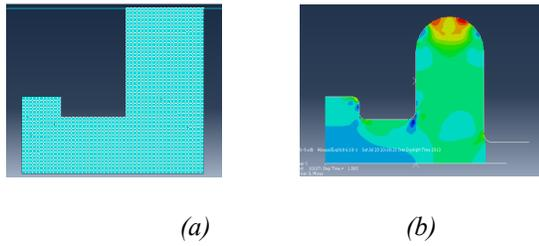
Figure 2. A view of forging process. (a) preform shape, (b) final product
