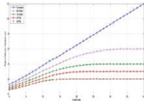
Fig. 3. Mutual information curves under FSA compared to channel capacity under ZMCSCG for 32 subcarriers at 10mW
