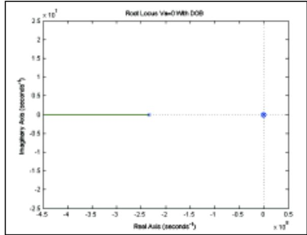
Figure 9 : Root locus plot for  $\omega_{ref}=0$ , with DOB
