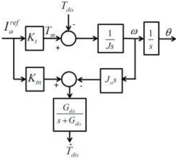
Figure 4: Control block diagram of disturbance observer
