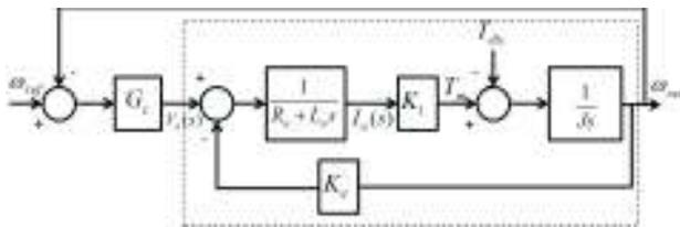
**Figure 2 : PID based velocity controller**
