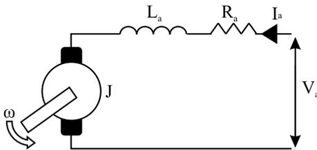
**Figure 1: Electrical model of a DC motor**
