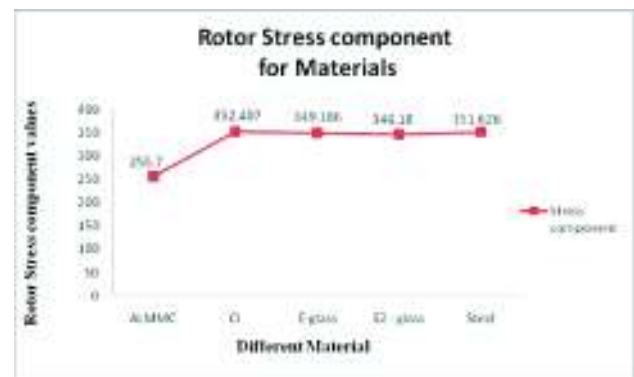
Figure 5.2 (b): Rotor Stress Component for Different Material
