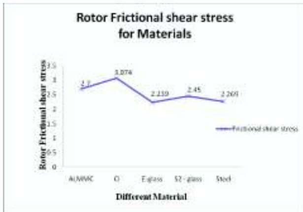
Figure 5.2 (d): Rotor Frictional Shear Stress For Different Material.
