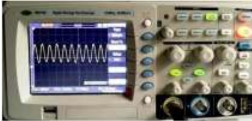
Figure 7: Wave form Observed at the LED1
