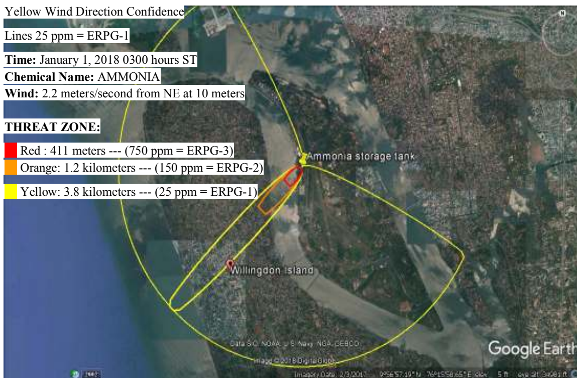
Figure 2: Ammonia toxicity impacted area (represent the largest impact observed for night time)
