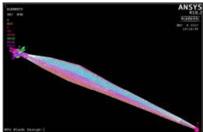
Figure 16: Fixing the ends of blade for extraction of Modes during Buckling Analysis
