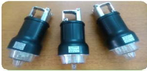
Figure 1: Fault passage indicators
