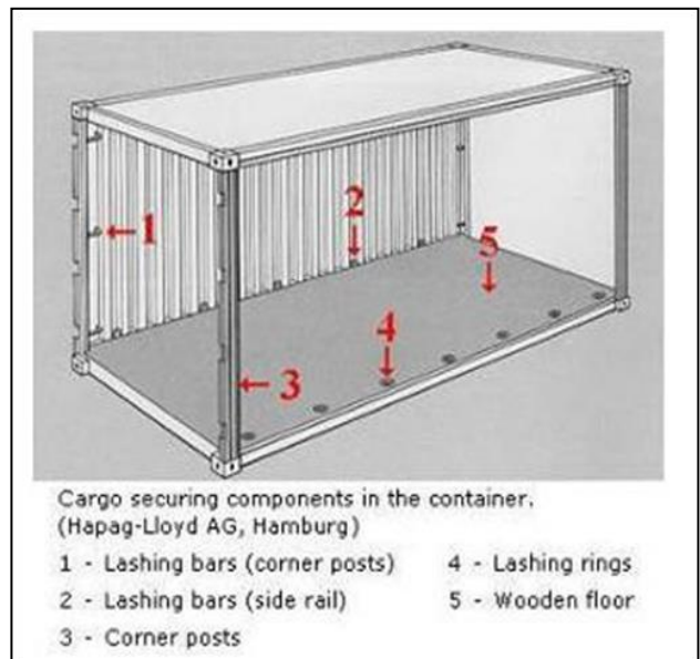
Figure 9 Composition of Shipping Container
