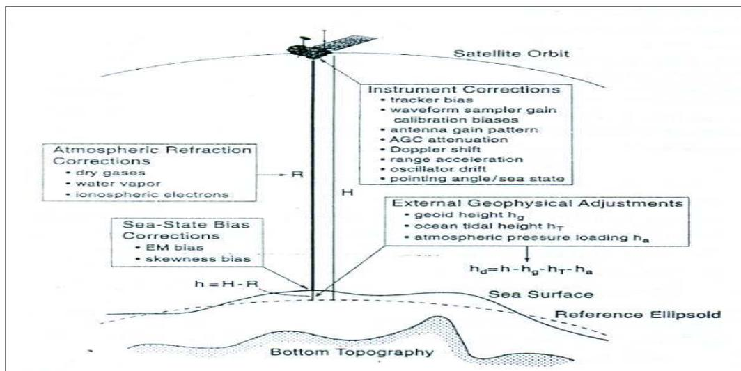
Figure 2: Schematic diagram of the range measurement by an altimeter
