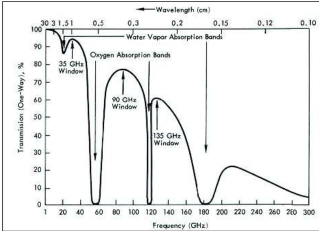
**Figure 1: Percentage transmission of microwave through the earth’s atmosphere, along the vertical direction, under clear sky conditions**
