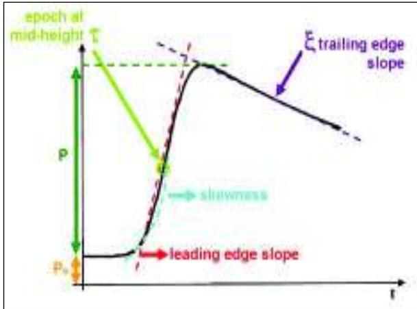
**Figure 3: Basic schematic outlines of a return echo over the ocean**
