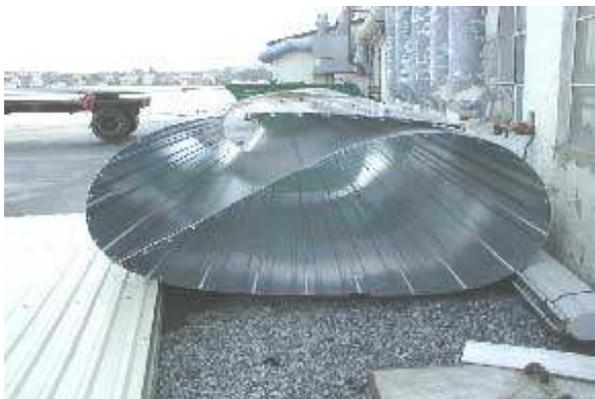
Fig. 4: Prefabricated FSW panel for a catamaran sidewall, rolled for road transport
