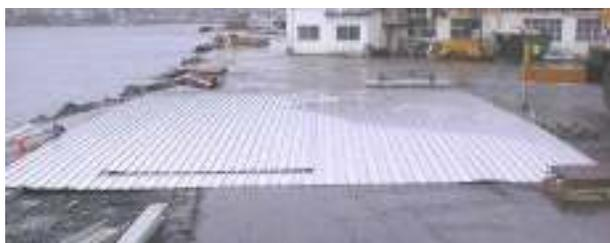
Fig. 5: Prefabricated FSW panel for a catamaran sidewall, straight panel for ship transportation at Marine Aluminium in Haugesund in Norway
