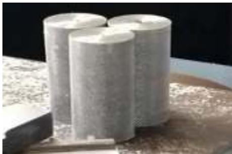
Fig. 8. Knurled rollers for four point bending test
