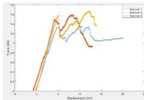
Fig. 14. Displacement vs load delamination Results
