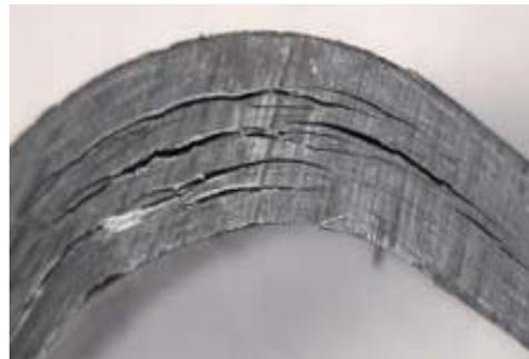
Fig. 13. Delamination of CFRP composite specimen
