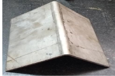
Fig. 3. V- Shaped stainless steel tool
