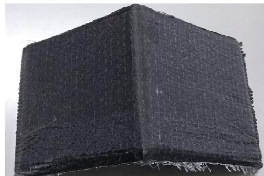
Fig. 5. Composite specimen after curing
