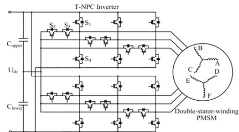
Fig. 1. Configuration of T-NPC double-stator winding PMSM drive
