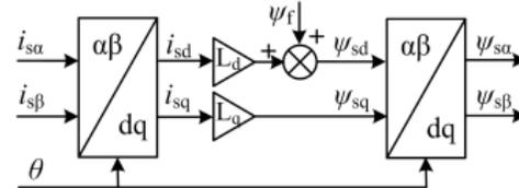
Fig. 4. Calculation of stator flux based on current model.
