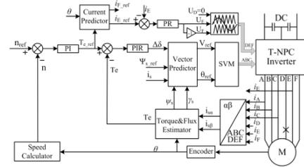
Fig. 3. Block diagram of hybrid fault tolerant control for T-NPC double-stator-winding PMSM drive.
