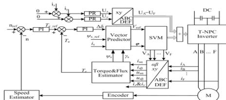
Fig.2. Control diagram of the proposed VSD based DTC for T-NPC three-level inverters fed double-stator-winding PMSM
