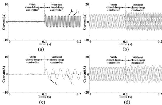
Fig. 6. Simulated performance of closed-loop current controller on x-y subspace: (a) x-y current components with 5th harmonics in back EMF; (b) stator currents with 5th harmonics in back EMF; (c) x-y current components with asymmetric resistor in phase A; (d) stator currents with asymmetric resistor in phase A.
