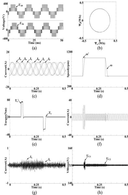
Fig. 5. Simulated performance of drive under normal condition: (a) inverter output voltage waveform; (b) stator flux trajectory; (c) stator currents; (d) rotor speed; (e) torque; (f) stator currents; (g) harmonics on x-y subspace; (h) DC link capacitor voltages.
