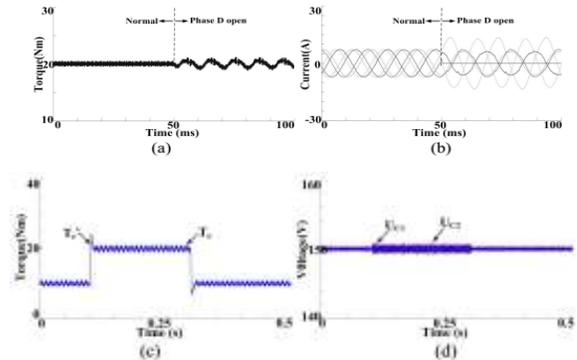
Fig. 7. Simulated performance of drive with standard SVM-DTC under one-phase open-circuit fault: (a) torque; (b) stator currents; (c) torque during transient process; (d) DC link capacitor voltages during transient process.
