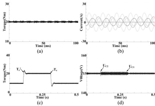
Fig. 8. Simulated performance of drive with proposed fault tolerant control under one-phase open-circuit fault: (a) torque; (b) stator currents; (c) torque during transient process; (d) DC link capacitor voltages during transient process.
