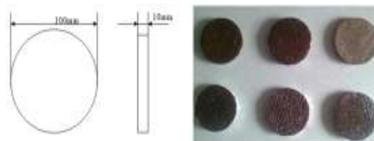
Figure 1: Specimen for thermal conductivity test.
