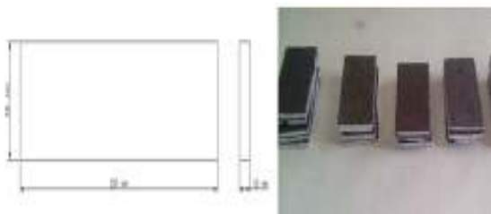
Figure 2: Specimens for thermal expansion test
