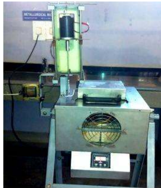
Figure 1: Shows the stir casting set up
