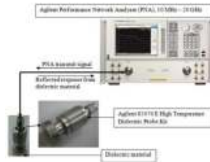
Fig. 3. Dielectric Properties measurement with Agilent 85070B High Temperature Dielectric Probe Kit measurement system setup
