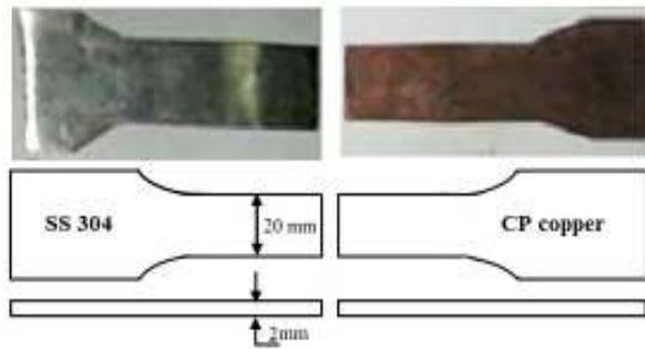
Figure 1: Orientation of butt joint
