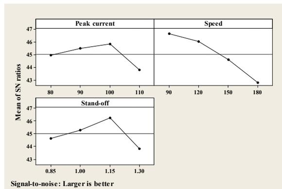
Figure 2: Main effect plot for output response tensile stress
