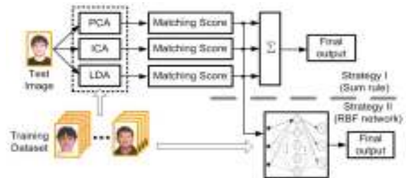
Figure 2: Schematic design of a hybrid system PCA, LDA and ICA
