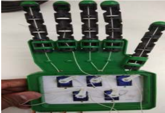
Fig. 4. Helping hand with Servo motors
