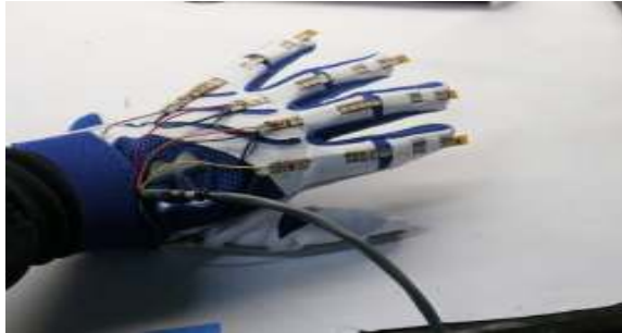
Fig. 3. Helping hand with flex sensors
