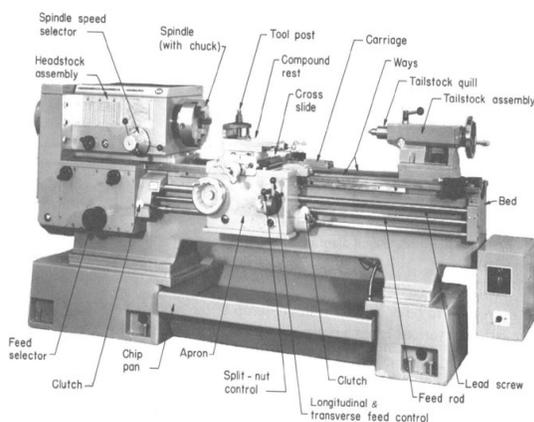
The work may be held on one or by both its ends. Holding the work by one end involves gripping the work in one of several types of chucks or collets. The spindle is mounted in the lathe's "headstock," which contains the motor and gear train that makes rotation possible. Directly across from the headstock on the lathe is the "tailstock." The tailstock can hold
