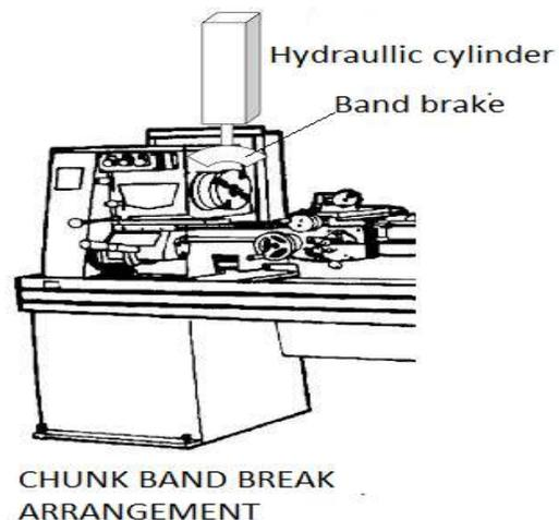
In case of turning, chunk is free to rotate about its axis but when auxiliary operations are carried out chunk is locked by band brake which is mounted above the the chunk & In conjunction with hydraulic ram fitted to it & transmit movement to shoe to engage with chunk. This causes braking action on chunk.
