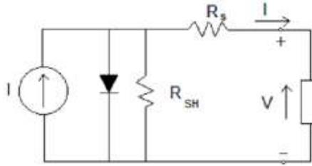
Fig.4. Single diode model of a PV cell
