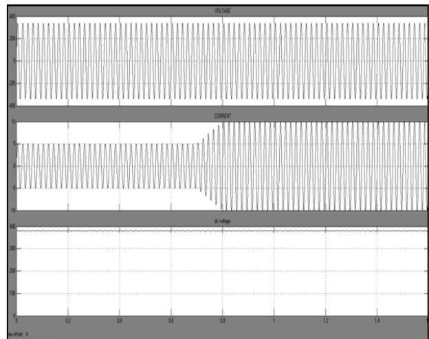
Fig.19. Simulation results of proposed system with an irradiance variation followed by a battery charge
