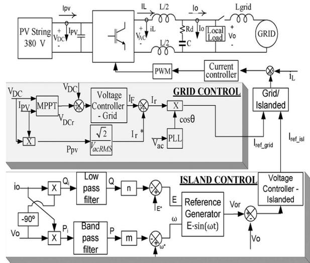
Fig. 9. Control structure of the PV inverter.
