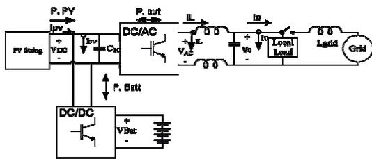
Fig.8. Block Diagram Of The PV System Under Study
