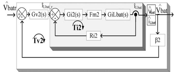
Fig.12. DC/DC converter control loops in grid-connected operation.
