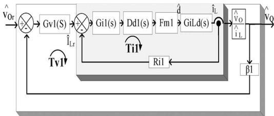
Fig.13. Inverter control loops in islanDED operation.
