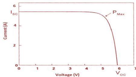
Fig.5. I-V characteristics of a solar panel
