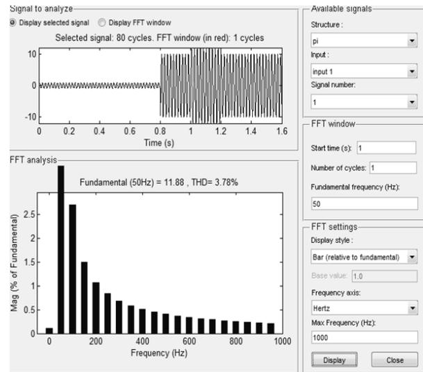
Fig:23. THD of islaneded mode to grid connected mode with PI controller
