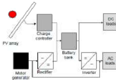
Fig.3. Schematic Diagram Of Hybrid System Incorporating A Photovoltaic Array And A Motor Generator (E.G. Diesel Or Wind).
