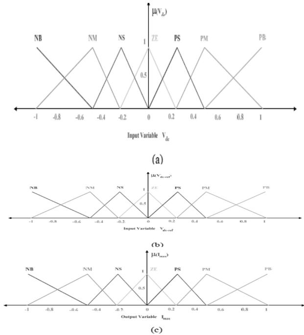
Fig.16. (a) Input Vdc normalized membership function; (b) Input Vdc-ref Normalized Membership Function; (c) Output Imax Normalized Membership Function.
