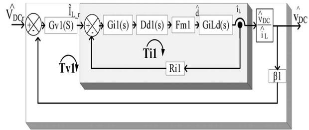
Fig.11. Inverter control loops in grid-connected operation.
