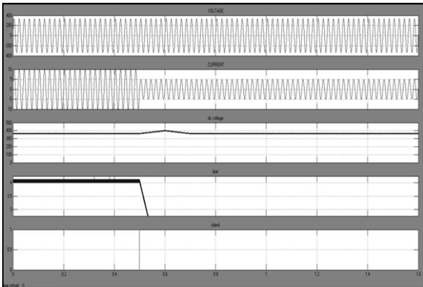
Fig. 25 Transition from islanded mode to grid-connected mode.
