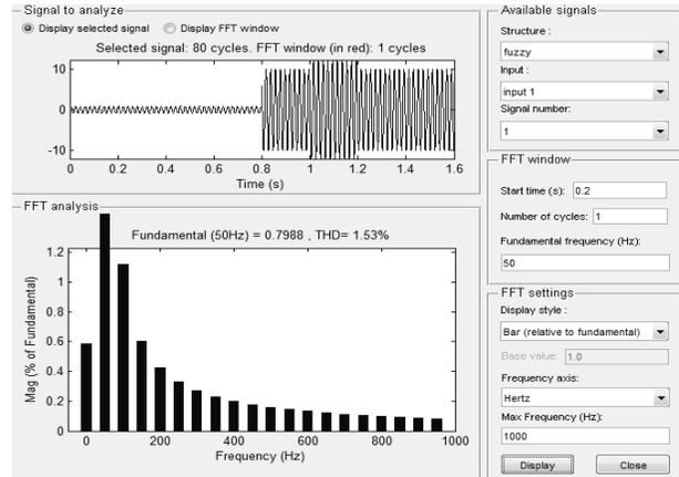
Fig: 27. THDV of islanded mode to grid connected mode with fuzzy controller.
