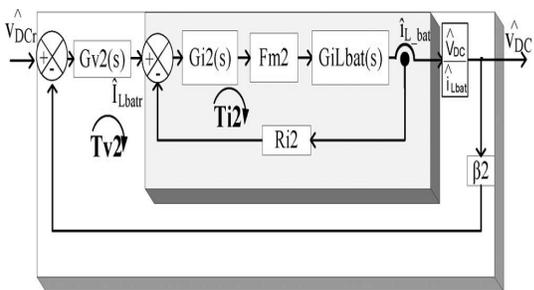
Fig.14. DC/DC converter control loops in islanDED operation.
