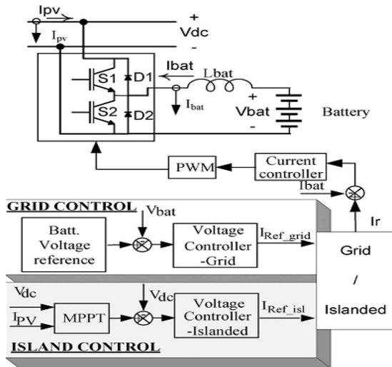
Fig.10. DC-DC converter schematic and control structure.
