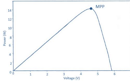
Fig.6. : P-V characteristics curve of photovoltaic cell
