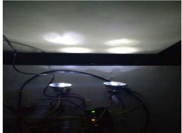
Fig. 6. Appearance of the high beam condition on the wall
