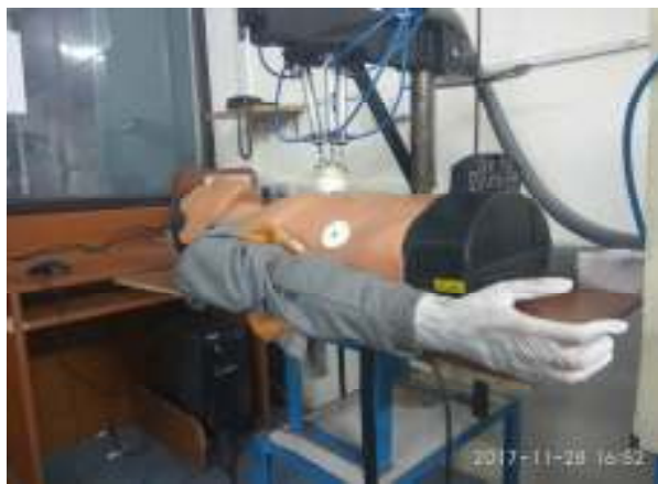
Fig.3 Experimental setup of Ambu manikin during CPR using mechanical compressions
