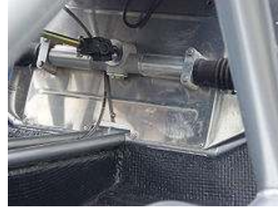
Enclosed steering rack in an automobile
