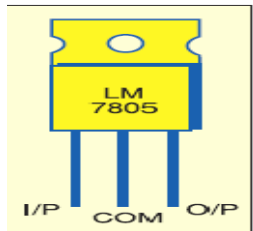
Figure 2.7(A): Voltage Regulator
