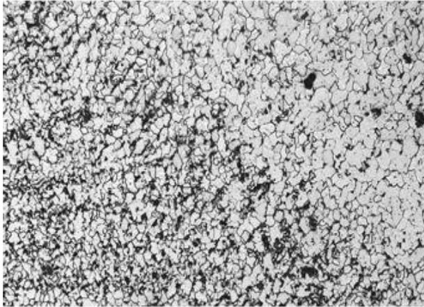
**Figure 1a: Weld 1-HAZ@200X**
