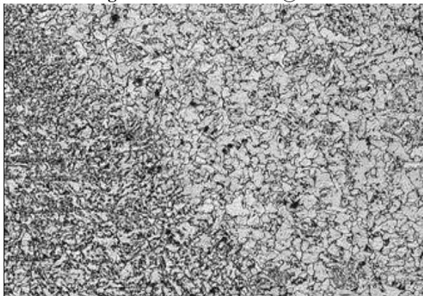
**Figure 1b: Weld 2-HAZ@200X**
