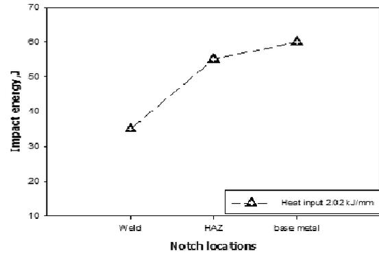
Figure 3: Notch Toughness, heat input at 2.02 kJ/mm
