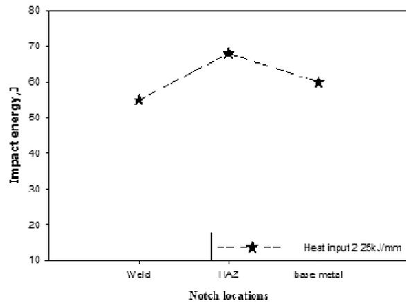
Figure 4: Notch toughness, heat input at 2.25 kJ/mm
