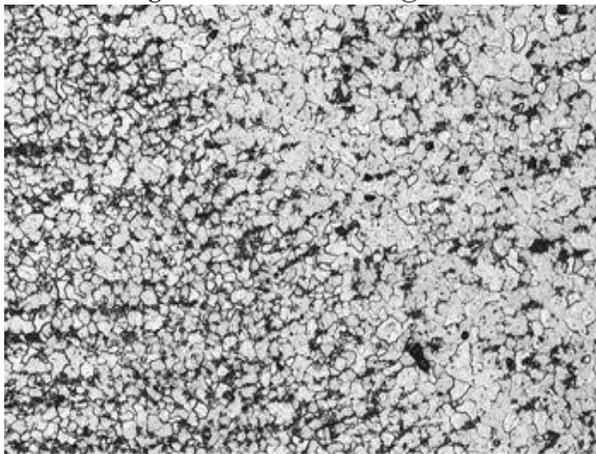
**Figure 1c: Weld3- HAZ@200X**
