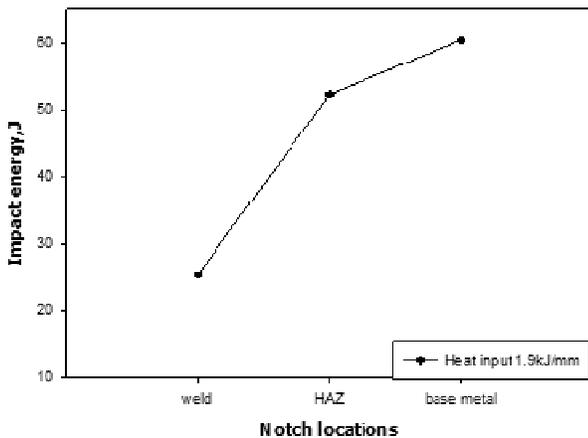
Figure 2: Notch toughness, heat input at 1.9kJ/mm
