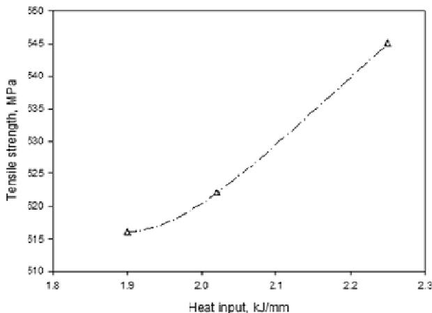
**Figure 6: Strength vs Heat input**
