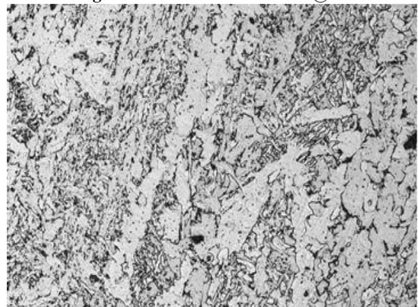
**Figure 1e: Weld2- Weld metal@200X**
