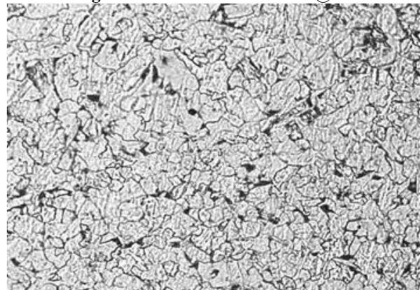
**Figure 1f: Weld 3- Weld metal@200X**
