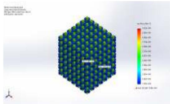
**Figure 10: Von mises Stress distribution on Model M1 Scaffold Structure**
