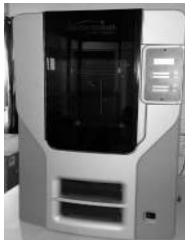
Fig 3. STRATASYS Dimension 1200 E S 3- D Printing machine (F D M)
